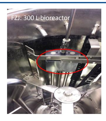
Monitoring gradients by multi-position sensor (pH, pO<sub>2</sub>) in 100 and 300 L bioreactors at TU Berlin and FZ-Jülich
