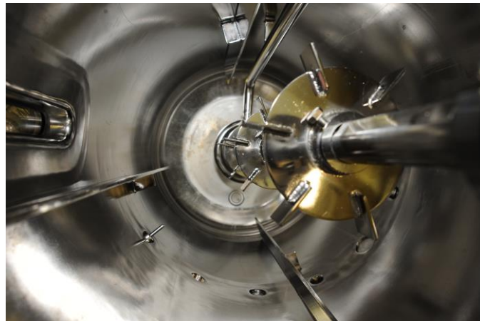
Figure 1: Inside of pilot scale bioreactor for microbial bioproduction processes showing baffles on the inside wall, aeration device at the bottom and the stirrer shaft in the middle with mounted stirrer devices
